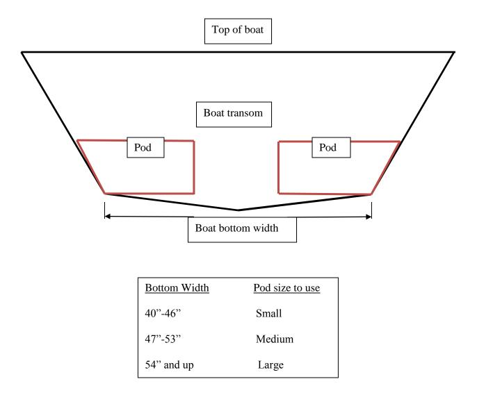
16" between the pods is normally the very minimum amount required to be able to turn the motor without interference. Some Surface Drive motors may require more.
