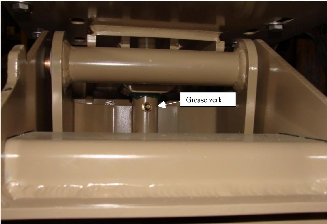
Lubricate motor pivot every 5 hours of operation using a quality marine grease.
