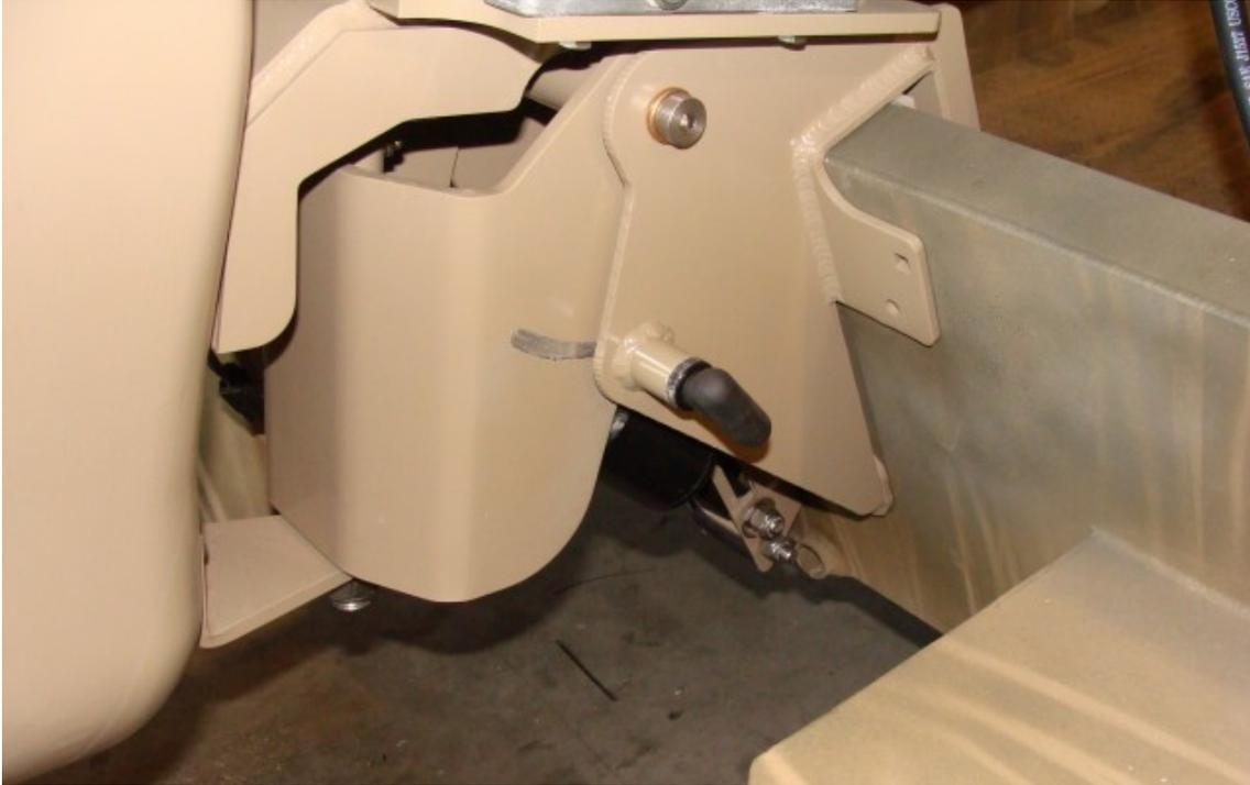
When trailering the motor make sure it is trimmed all the way up and the travel lock is locked into place. There should be no movement in the motor. The tilt and trim should be in the up position when trailering to avoid any movement of the motor. Failure to do so can result in severe damage to the frame and is not covered under warranty.
