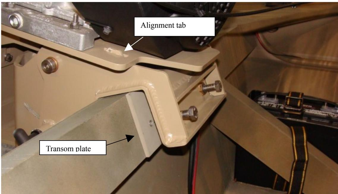
When installing the motor on the boat the transom plate should be installed between the boats transom and the transom bolts.
