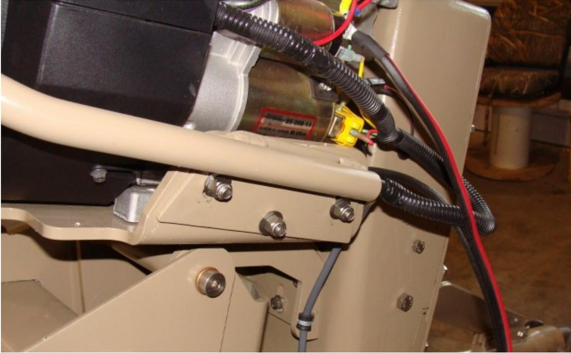
Install handle on the motor with the three bolts, nuts and washers as shown above. The bolts should be snug but allow the handle some movement up and down. This helps to absorb the shock from hitting obstructions.
