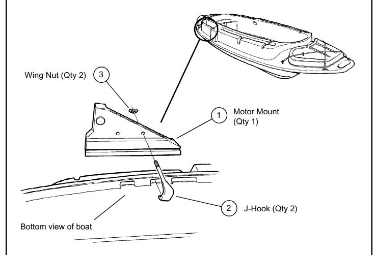
Note: Designed for the use of an electric trolling motor or a small out-board on your Stealth 1200 or 2000.
