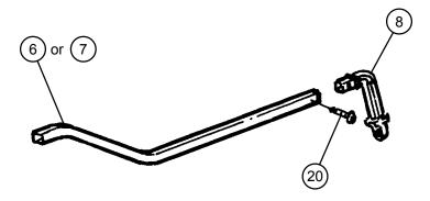
12. Slide the bent outer bar (Item 6 and Item 7) through the sleeve of the canvas cover (Item 13) until the hinge elbow (Item 8) reaches the hinge bracket (Item 4). (Be sure to have the correct bent outer bar for the head and foot). Repeat on the other side.
