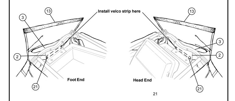
16. Assembly is complete. Open main bar assemblies to enter in and out of the Predator. Outside canvas cover is equipped with nylon loops for securing vegetation for a more realistic effect if desired.
