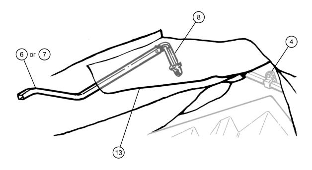
13. Attach the hinge elbow (Item 8) to the hinge bracket (Item 4) with 1/4 x 1 1/4 bolts (Item 15) and 1/4 nylon lock nuts (Item 17). (Be sure to have the correct bent outer bar for the head and foot). Repeat on the other side.
