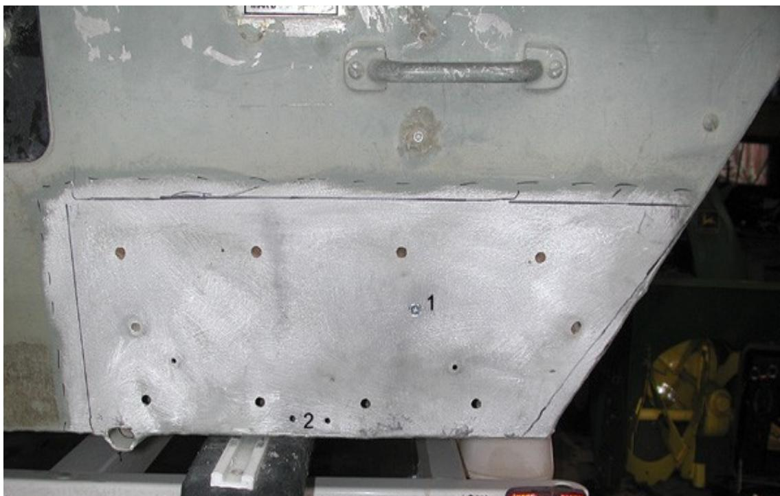
2. The pods should be welded on so that they are tipped up at the back about  $\frac{1}{2}$ " for optimum performance. The boat may porpoise if they are tipped up more than that.
