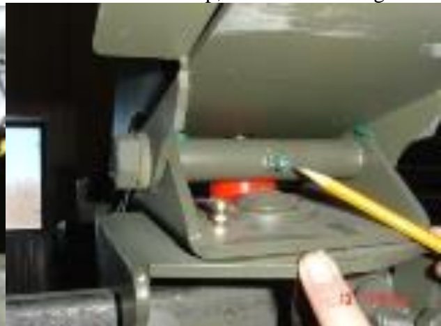
Grease Zerks for up, down and turning
