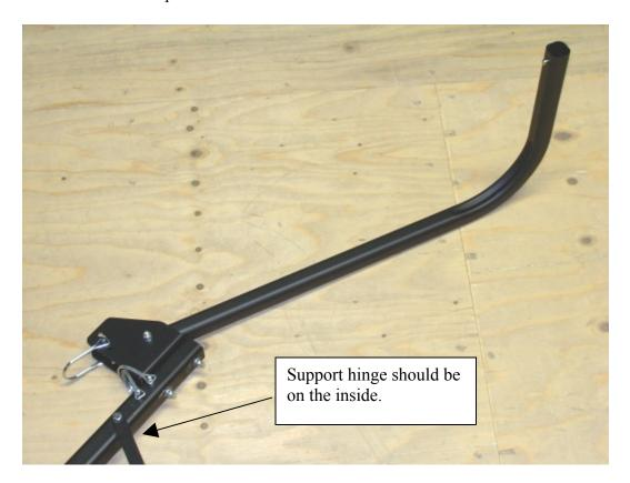
4. Assemble the three large center bars. The longer piece with the two flared ends will be in the middle and the other two pieces will slide into place, one from each end. Use two self tapping screws at each joint to reduce the amount of movement in the pole. If you need to be able to disassemble the poles so the blind is a more compact size then do not install the self tapping screws.
