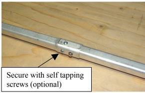
6. Attach the small elbow to the small center bar as shown. Attach an elbow on each end.
