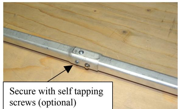
6. Attach the small elbow to the small center bar as shown. Attach an elbow on each end.
