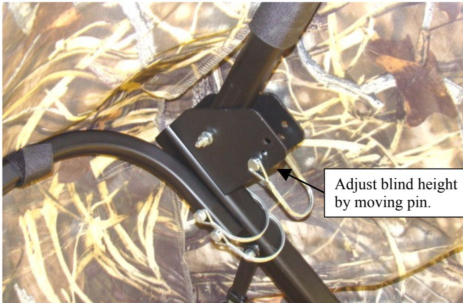
15. To lock the blind in one position so it cannot be flipped open first determine the proper height for your situation. Next drill a hole through the main support pole so the pin will fit through it. The pole should be lined up with one of the three holes in the hinge bracket when the hole is drilled.
