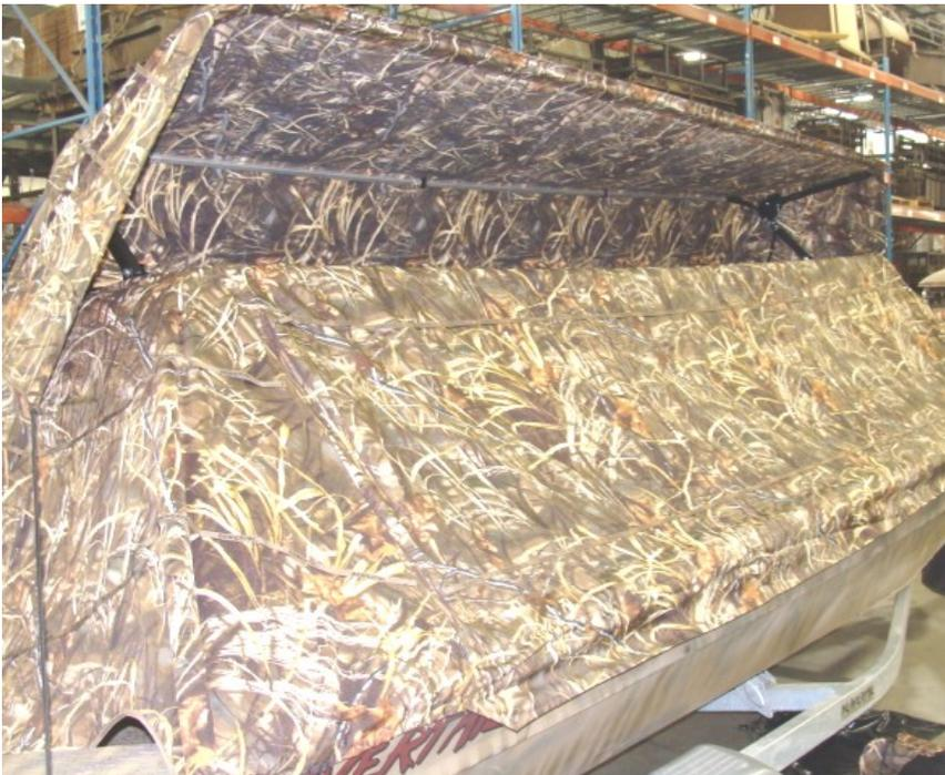
14. The front opening or height of the blind may be adjusted by changing the position of the pin in the hinge bracket. There are three holes to adjust the blind from low to high.
