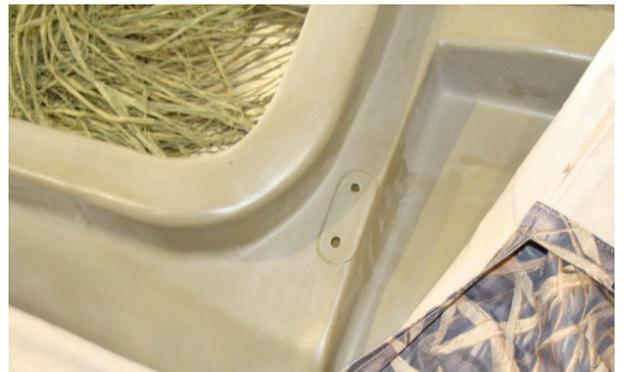
2. Bolt the brackets onto the boat using the 10-24 x 3/4" bolt, washers and nylock nuts. Be sure to attach so that the screw is to the outside.
