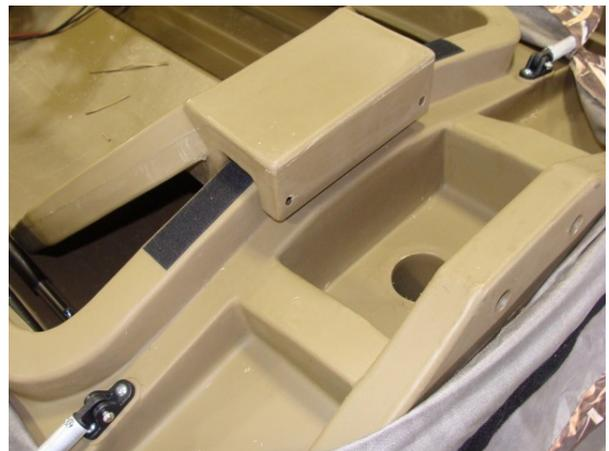
2. Mark a spot 1" up from the bottom of the backrest bracket and 1/2" in from the side of the bracket. Repeat on the other end of bracket. Drill a 5/16" hole through the backrest bracket and all the way through the lip of the cockpit, both the outside and the inside. The holes will be angled slightly downward. Push one of the 5/16" detent pins into the hole to lock the backrest in place. Drill the second 5/16" hole.
