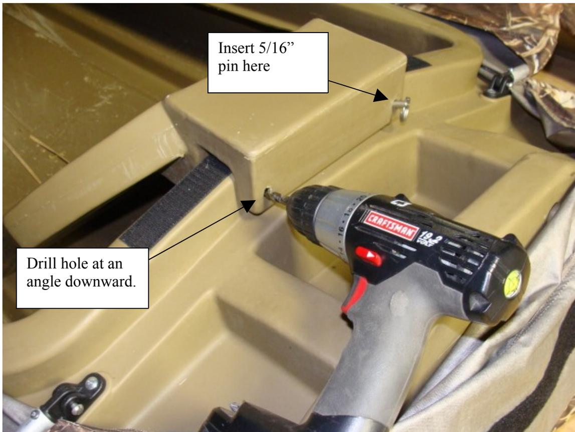
3. Insert the second 5/16" pin into the last hole. The backrest should now be fully locked into place.
