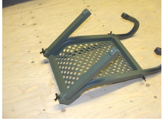
3. Insert base adjustment poles into the main bottom poles and tighten in place with the thumb screws. These poles may be adjusted in or out to fit a particular boat.
