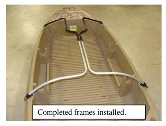
7. Install support brace as shown. Loop bottom seat straps around the tube and latch. Loop top seat straps around the boat handle at the boat front and latch. Adjust as necessary for a comfortable fit.
