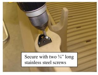
3. Attach door frame to bracket at center of boat using the locking pin and place 2 x 4 across the boat to help support it. Attach another bracket to the other end of the door frame and align it on cockpit edge as shown. Mark location and secure bracket with two 3/4" stainless steel screws.
