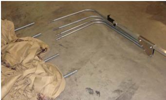
6. Attach the elbows to the straight center sections using the  $\frac{1}{4}$  x 1  $\frac{1}{4}$  bolts and nylock nuts. Start with the top elbow and the top center section and work your way down . Repeat on the other side.
