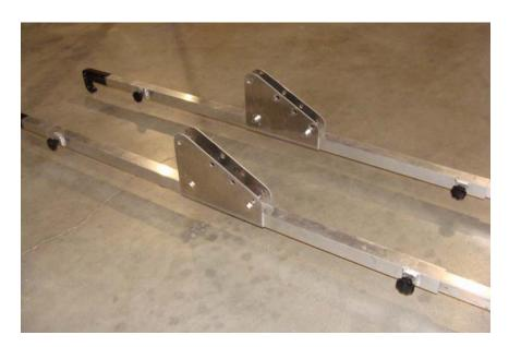
2. Fasten the four elbows to the support hinges using the  $3/8 \times 2$  bolts, plastic washers and the 3/8 nylock nuts.
