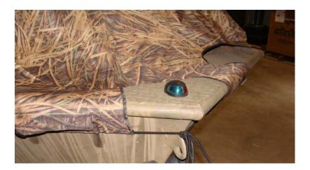
9. Attach the travel boot by first folding the ends of the blind towards the center so all of the material may be covered when traveling. Also attach the travel straps around the elbows and the main support bars.
