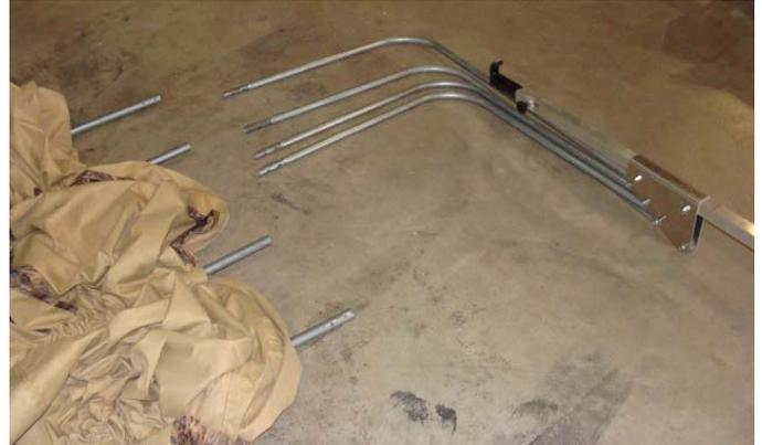
6. Attach the elbows to the straight center sections using the  $\frac{1}{4}$  x  $1 \frac{1}{4}$  bolts and nylock nuts. Start with the top elbow and the top center section and work your way down. Repeat on the other side.
