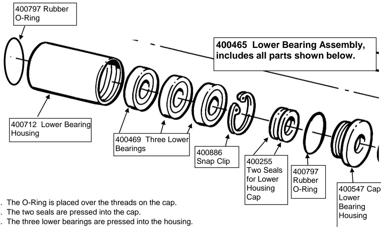
1. The O-Ring is placed over the threads on the cap.
