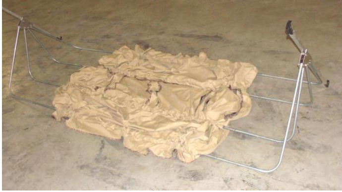
All eight elbows attached.
