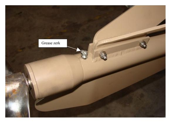
Lubricate the prop drive every 100 hours or once per year. Fill the tube until the grease comes out of the inspection hole.
