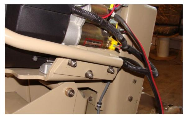
Install handle on the motor with the three bolts, nuts and washers as shown above. The bolts should be snug but allow the handle some movement up and down. This helps to absorb the shock from hitting obstructions.
