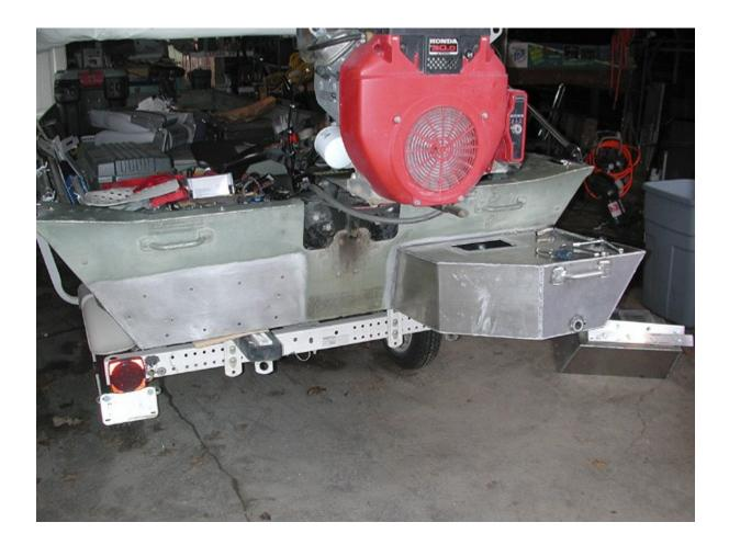
Apply a liberal amount of sealant to the surface of the pod (around each hole and near the outer edges of the pod). Secure the pod to the transom with two bolts. Apply the sealant to each reinforcing strip and install them using the eight main mounting bolts. Work quickly to get all of the bolts in place and tightened before the sealant becomes too stiff to adhere properly. Once the first pod is in place the second pod may then be mounted onto the boat by repeating the process.
