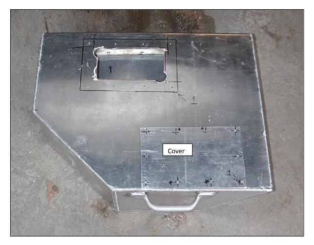
1. Cut an access hole (#1) in the top of each pod. After the pods are installed, a cover (not included) is fastened over each access hole with sealant and screws. Another option is to install an access hatch available from marine supply dealers. They can be either round or rectangular. This provides a clean professional look.
