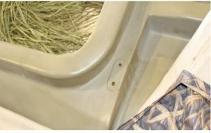
2. Bolt the brackets onto the boat using the  $10-24 \times \frac{3}{4}$ " bolt, washers and nylock nuts. Be sure to attach so that the screw is to the outside.
