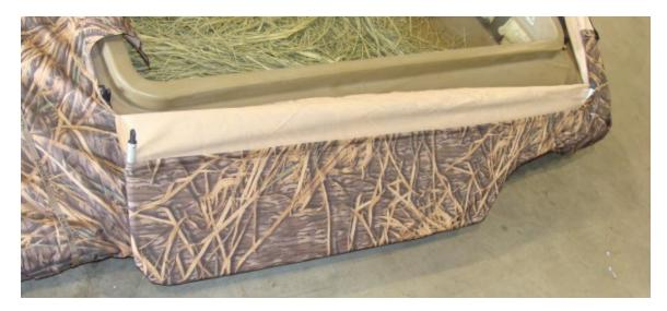
6. Attach the door frames to the hinge brackets on the boat using the screw that is with the bracket. Do that at all four locations.
