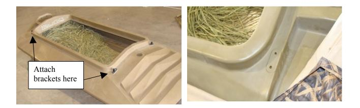
2. Bolt the brackets onto the boat using the 10-24 x  $\frac{3}{4}$ " bolt, washers and nylock nuts. Be sure to attach so that the screw is to the outside.
