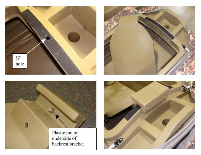
2. Mark a spot 1" up from the bottom of the backrest bracket and  $\frac{1}{2}$ " in from the side of the bracket. Repeat on the other end of bracket. Drill a 5/16" hole through the backrest bracket and all the way through the lip of the cockpit, both the outside and the inside. The holes will be angled slightly downward. Push one of the 5/16" detent pins into the hole to lock the backrest in place. Drill the second 5/16" hole.
