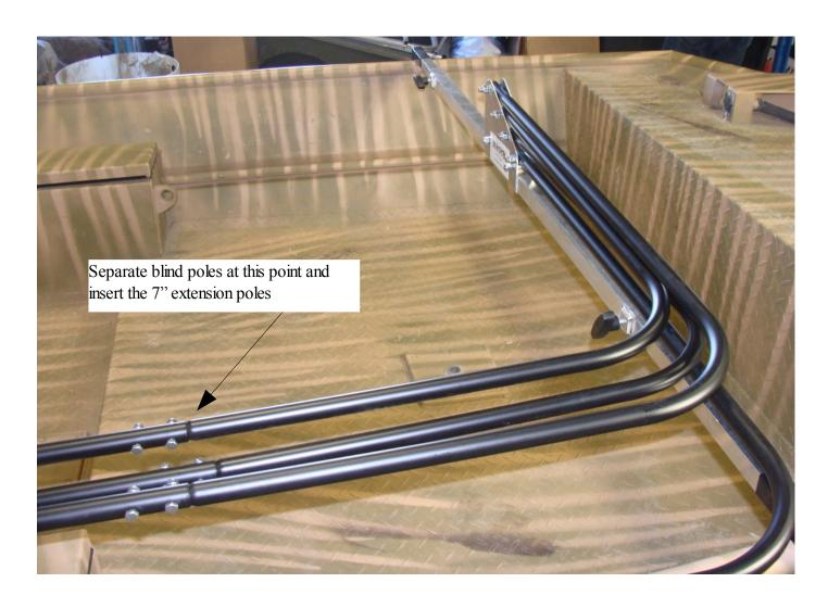
2. Insert the four extension poles in between the straight center sections and the elbows making sure to line up the holes. Tighten securely using the  $\frac{1}{4}$  x 1  $\frac{1}{4}$ " bolts.
