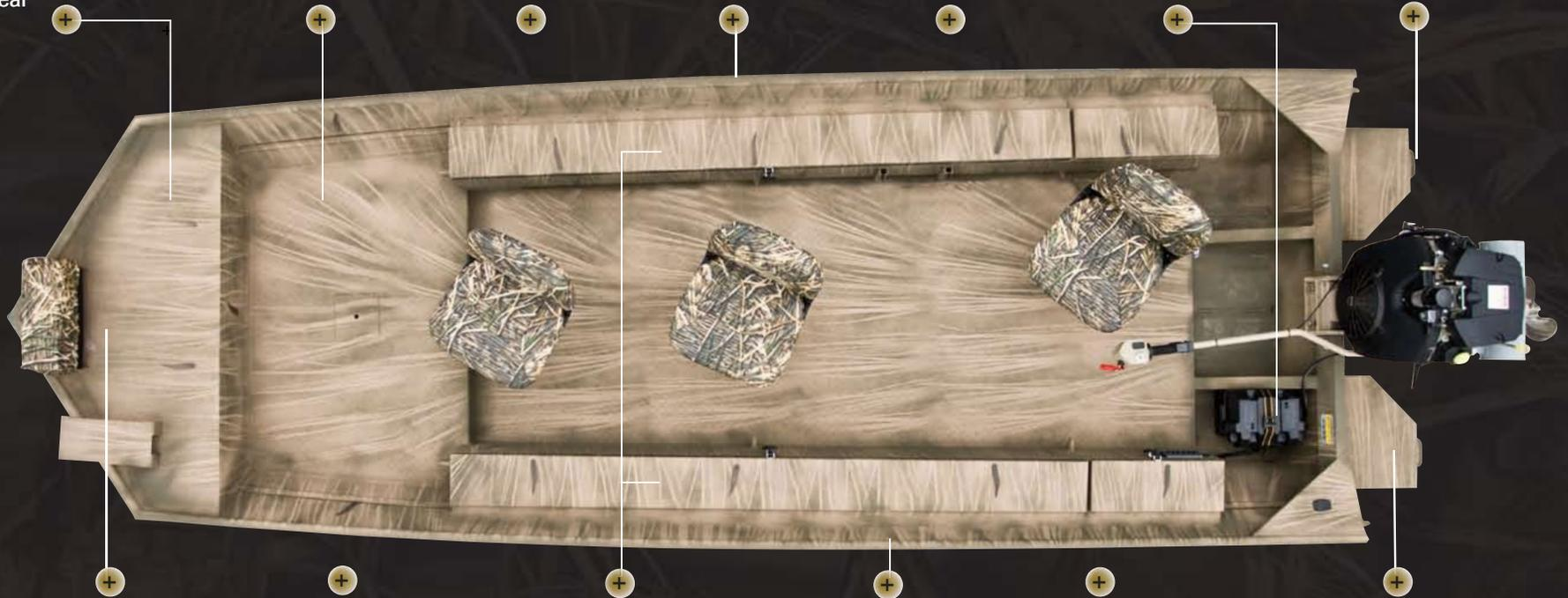
Foam-Filled Floor Front Deck and Pods for Extra Flotation and Load Off-Set
